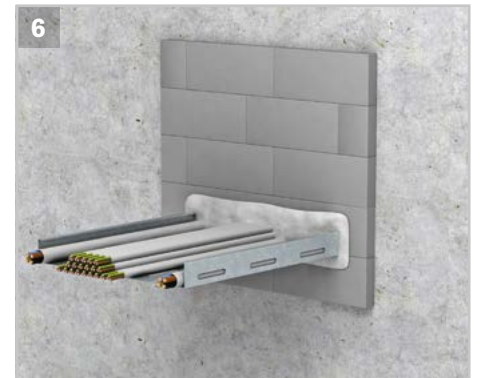
6 Check the sealing and apply the label.
