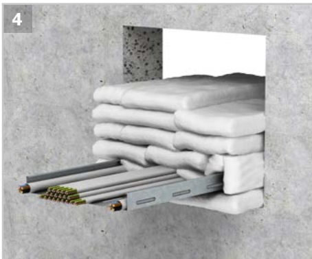
4 Coat the cables in the opening at a length of min. 10 cm with ROKU® FL Sealant and apply or cut additional bricks.
